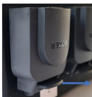
Figure 6: Pump cover flap in the locked position
