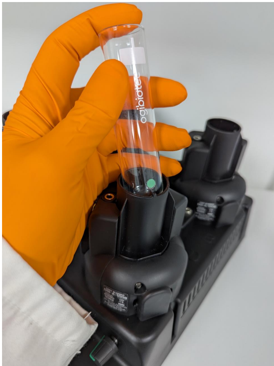
Figure 15: Correct alignment of oxygen sensor spot – Spot to notch in flask holder
