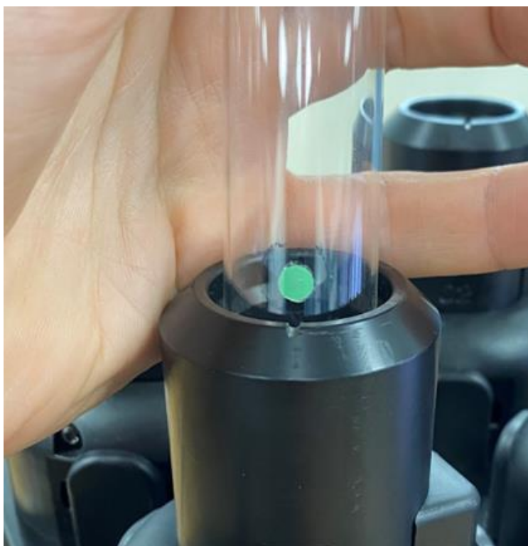
Figure 3: Correct alignment of oxygen sensor spot – Spot to notch in flask holder
