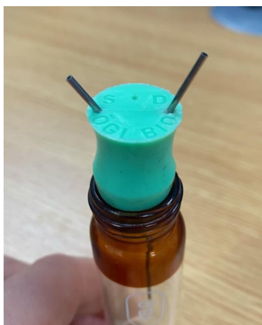
Figure 12: Culture flask with Bung. S – Addition from source. D – Removal to drain. Centre hole is a vent.
