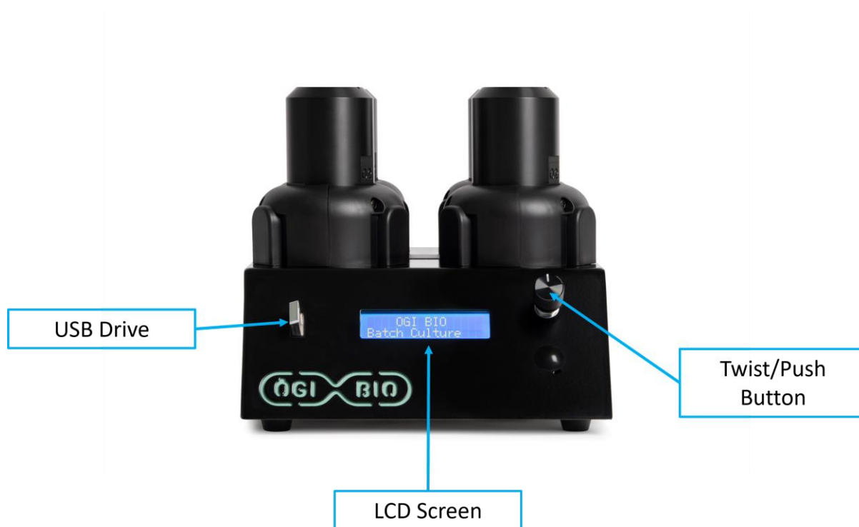
Figure 1A: The front view of the bioreactor with the key interface points labelled.
