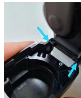
Figure 8: Line up latch and groove to reconnect pump cover
