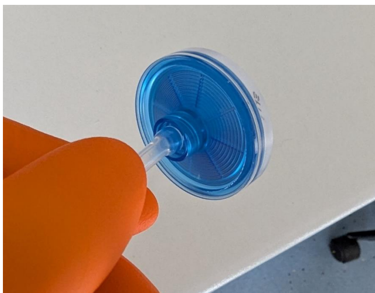
Figure 19: Attachment of sparging tubing over the small barb in the centre of the luer lock fitting. This is fiddly, however the tubing is quite flexible and will be secure once in place. Filters that have slip fittings on both sides are preferred when using the sparging system as they provide more flexibility in placement of the filter
