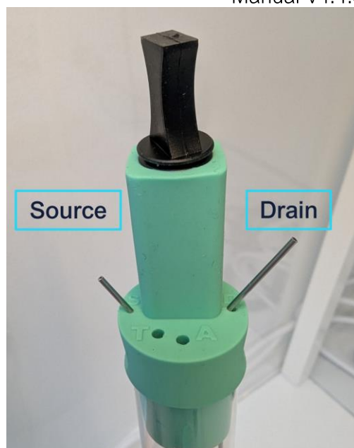
Figure 12: Ensure the input flask is connected to S (Source) and the output or waste flask is connected to D (Drain).
