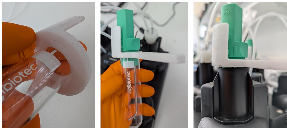
(a) (b) (c) Figure 21: Correct application of the spill guards to the top of the OGI3 culture flask. Note that the inset portion on the underside of the spill guard should line up with the marker on the culture flask. The bung may then be aligned with the same marker for complete alignment of the now guarded culture flask.
