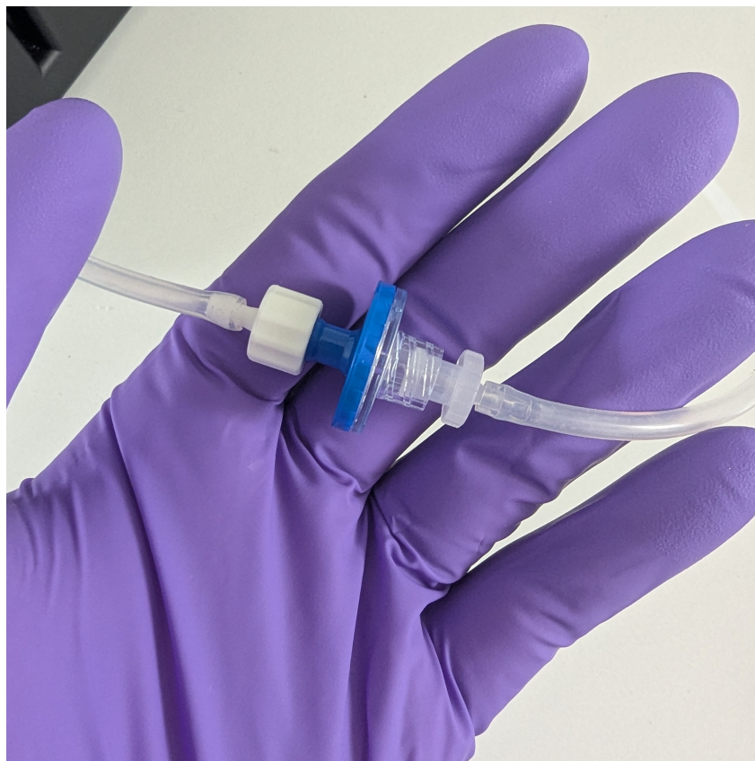
Figure 18: Hydrophobic filters are used to ensure safety of the pumps and sterilise the air input. These should be placed in the line prior to pre-humidifier flasks. Note that they will not prevent backflow, but will prevent liquid ingress into the sparging pumps.
