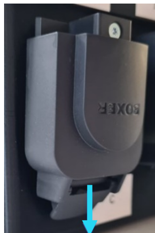
Figure 7: Pump cover flap in the open position
