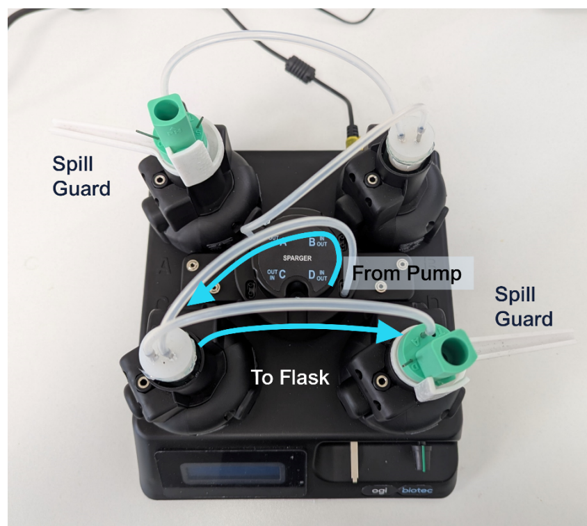
Figure 19: Sparging Module connected to culture flasks (green bungs) through pre-humidifier flasks (white bungs) with the route from Pump D to Flask D highlighted. Spill guards are fitted to the culture flasks.
