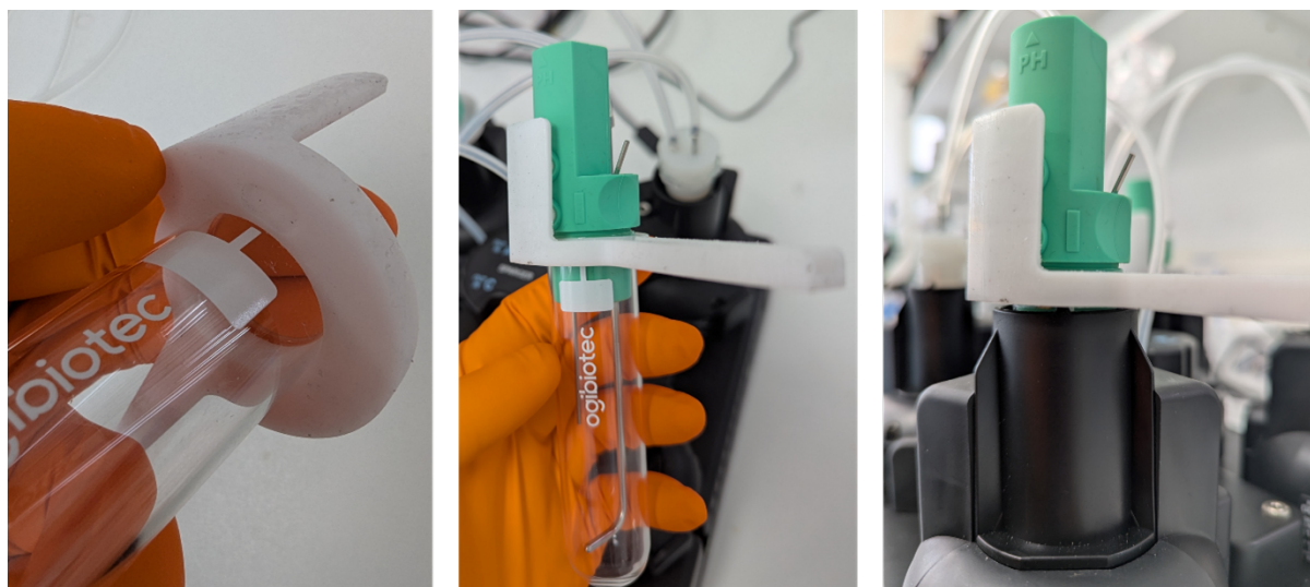
Figure 20: Correct application of the spill guards to the top of the OGI3 culture flask. Note that the inset portion on the underside of the spill guard should line up with the marker on the culture flask. The bung may then be aligned with the same marker for complete alignment of the now guarded culture flask.
