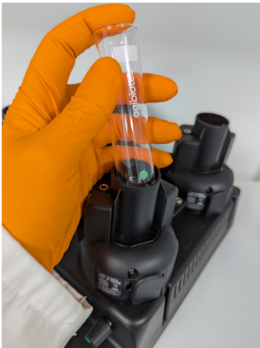
Figure 14: Correct alignment of oxygen sensor spot – Spot to notch in flask holder
