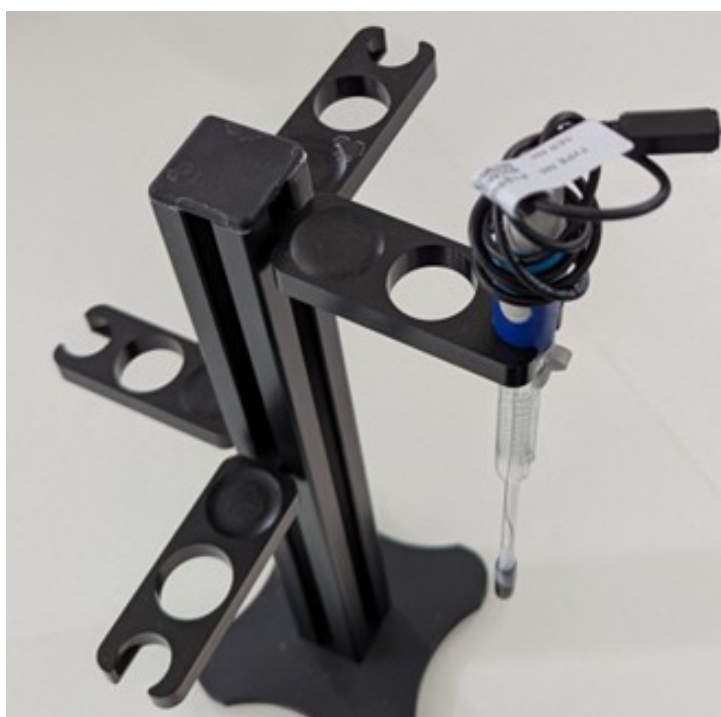
Figure 16: pH Probe held in the constructed pH probe holder
